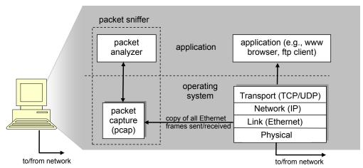
Figure 1: Packet sniffer structure
