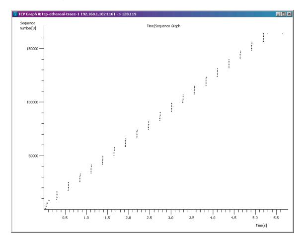
Here, each dot represents a TCP segment sent, plotting the sequence number of the segment versus the time at which it was sent. Note that a set of dots stacked above each other represents a series of packets that were sent back-to-back by the sender. Answer the following questions for the TCP segments the packet trace *tcp-ethereal-trace-1* in <u>http://gaia.cs.umass.edu/wireshark-labs/wireshark-traces.zip</u>
