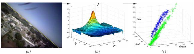
Fig. 3: (a) original image, (b) optimization criterion as a function of bank angle and pitch percentage and (c) resulting classification of sky and ground pixels in RGB space.
