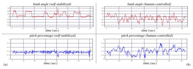
Fig. 5: (a) Bank angle and pitch percentage for a self-stabilized flight (sequence of level-flight and left-turn segments), and (b) bank angle and pitch percentage for typical human-controlled flight.
