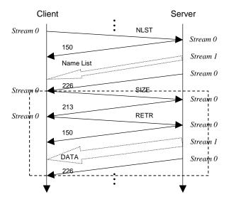
Figure 3: FTP over multistreamed SCTP timeline showing a multiple file transfer.
