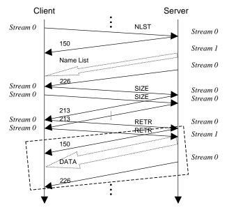
Figure 4: FTP over multistreamed SCTP with command pipelining timeline showing a multiple file transfer.
