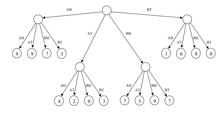
b) (7 points) Now assume that *there is no randomness* and the players simply can choose *any* of the four moves (*AH*, *AT*, *BH*, or *BT*). Apply the *minimax* algorithm to the tree below and explain which move the computer should make. As in part (a), assume it is the computer's turn to play.
