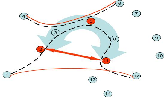
Fig. 1. Network topology with wormhole created by nodes 2, 5, and 11. Figure shows actual paths with dotted lines and advertised paths with solid lines. Actual path between nodes 1 and 12 is different from advertised path. Actual path and the advertised path between nodes 4 and 6 stays the same but overlaps with the wormhole tunnel.
