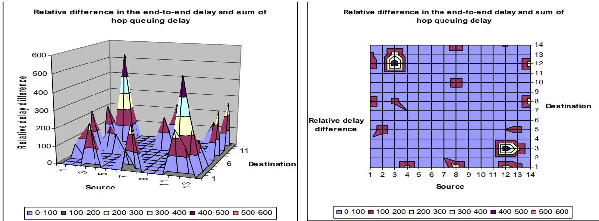
Fig. 4. Two different views of the relative difference in the end-to-end delay and sum of the queuing delay of the hops on various end-to-end paths. The relative difference is computed in this graph as  $((\text{end-to-end delay} - \text{sum of hop queuing delay}) / \text{end-to-end delay}) * 100$ .
