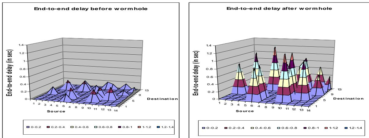
Fig. 5. End-to-end delay on various paths before and after the launch of wormhole attack.
