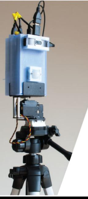
Thermporal: An Easy-to-Deploy Temporal Thermographic Sensor System to Support Residential Energy Audits
