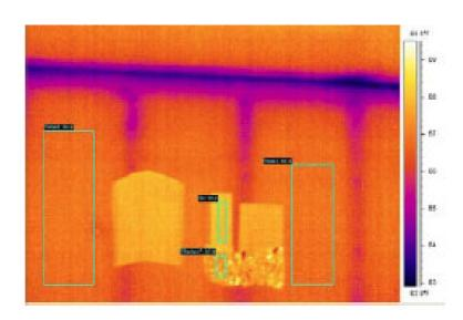
$$R - Value = \frac{\Delta T_{io}}{4\varepsilon\sigma T_m^3 \Delta T_r + h_c \Delta T_a}$$
