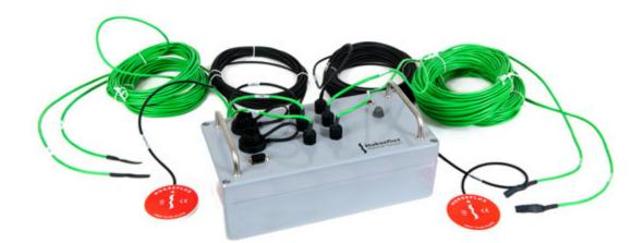
Direct Contact Methods: Heat Flux Sensors and Thermocouples
